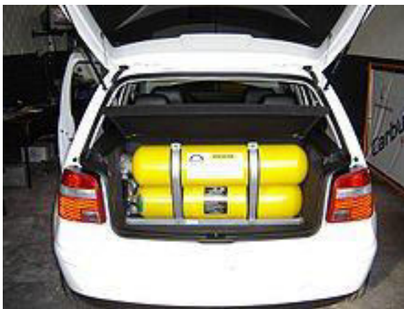
Position of Gas Containers
